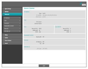
Change the network settings, enable FEN and security features, and control network bandwidth use.
