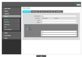
Frame Rate: Set the frame rate of image sesor. Selecting 30.00 ips limits the frame rate of images for streaming under Video > Streaming menu to 30.00 ips. Selecting 60.00 ips restricts some settings under Video > Streaming menu and disables the following functions: FTP upload, image attachment of emailing, and WDR.
